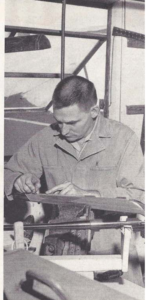
Weatherby gunsmith relieves wood in barrel channel to improve accuracy
