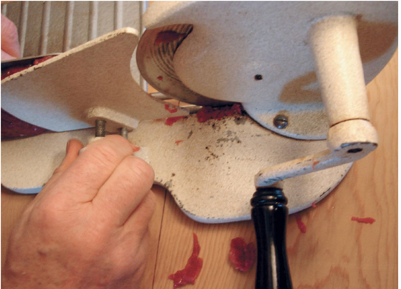
This hand slicer model has an adjustment knob on the side that allows you to increase or decrease the thickness of the meat slices.
